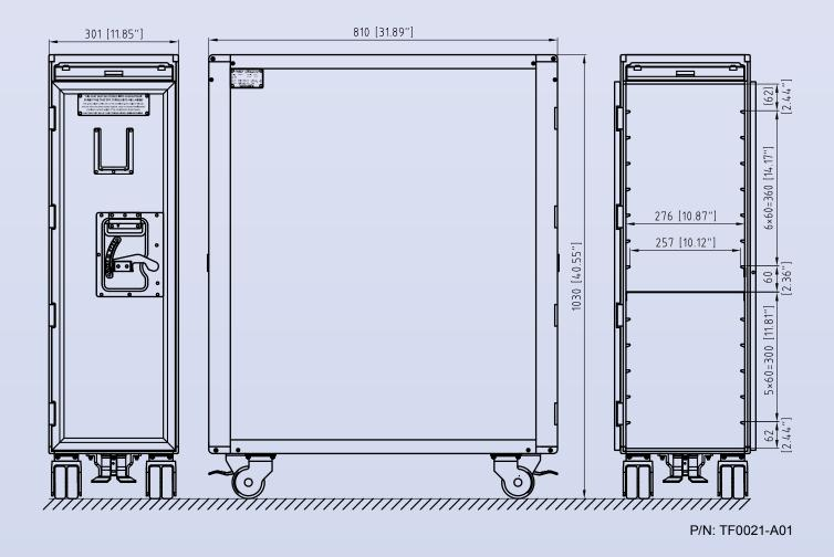
Lightweight Carts are made of high-grade aluminum alloys extrusions and sheets, stainless steel hardware, with approved insulation forms which meet all fire property requirements.
