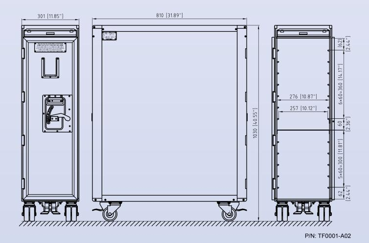
Reduced weight carts are made of high-grade aluminum alloy extrusions and sheets, stainless steel hardware, with approved insulation foams that satisfy all fire property requirements.
