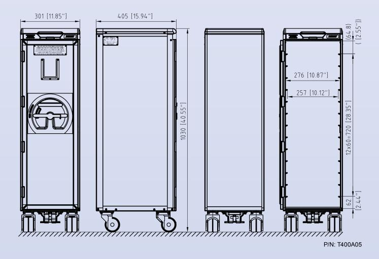
M-1 Series carts are designed to be more ergonomic while keeping its weight low and maintaining the same strength and robustness as the earlier generations. The new series provides better comfort and smoother operation by having rounder profiles and larger handles. Insulation properties have also been improved in the new design.
